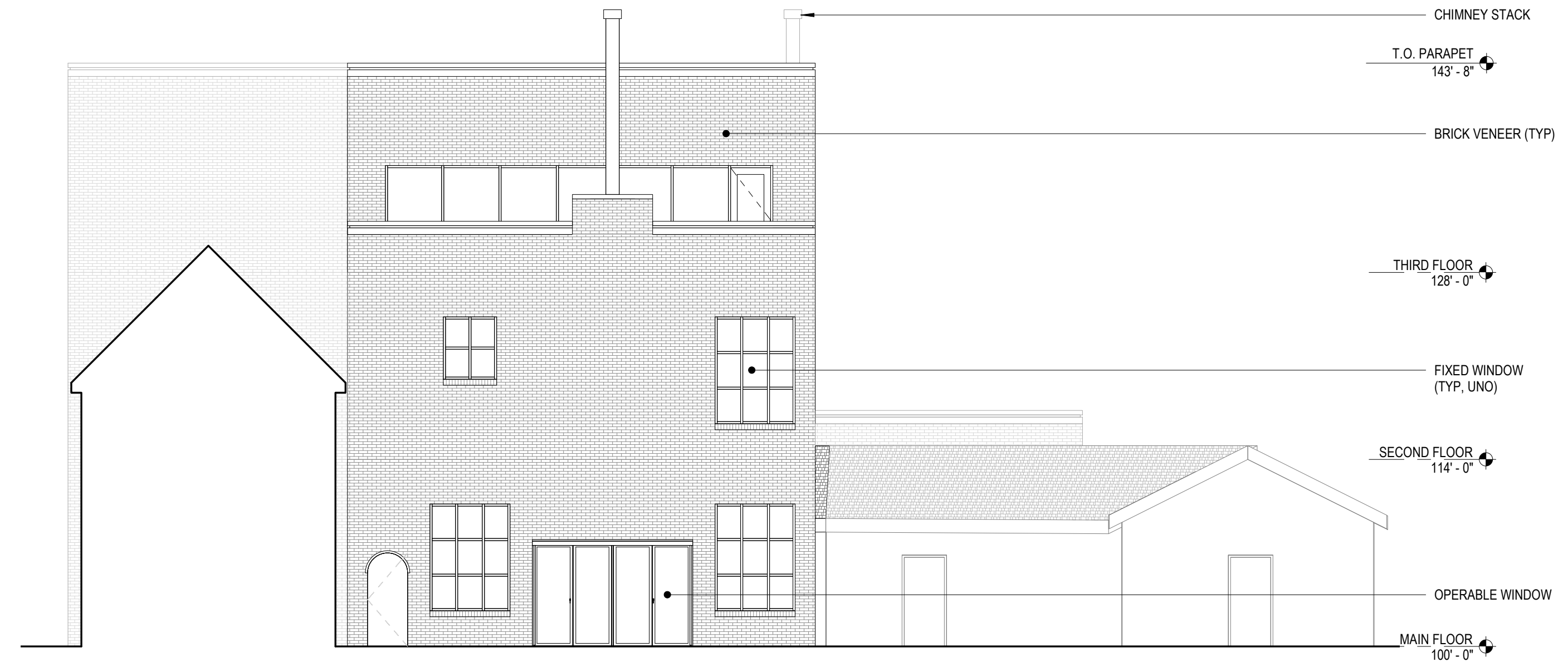
1 SOUTH EXTERIOR ELEVATION A201
